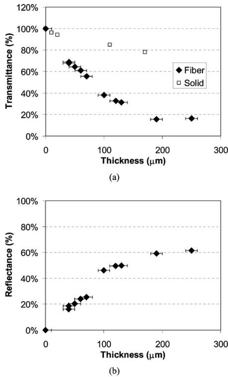
FIG. 9. (a) Hemispherical transmittance of ES PCL nanofiber mesh and solid PCL and (b) reflectance of nanofiber mesh for an unfocused femtosecond laser beam. Error bars indicate estimated  $\pm 10 \mu\text{m}$  accuracy in mesh thickness measurement.
