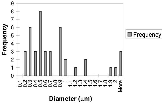
FIG. 1. Fiber diameter size distribution of ES-PCL meshes used in the experiments.
