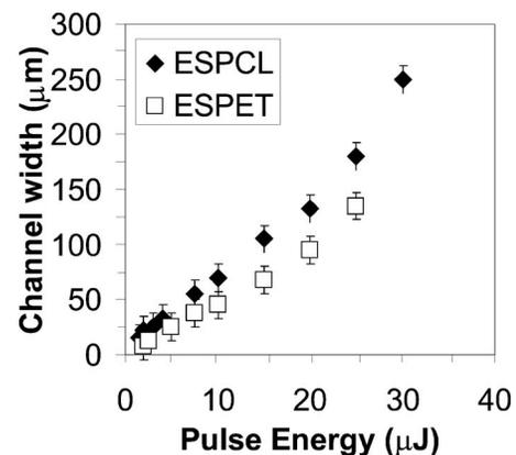
FIG. 3. Width of grooves machined in ES nanofiber meshes at various pulse energies using the 0.1 NA optic and speed of 20 mm/s. The groove width is generally much larger than the focus spot size of 6.4  $\mu\text{m}$ . Error bars indicate error in estimating groove dimension.
