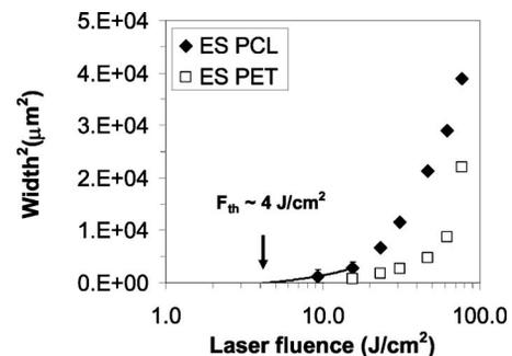
FIG. 8. Groove width squared of nanospun polymer vs fluence using the 0.1 NA optic showing nonlogarithmic behavior. The PCL ablation fluence threshold suggested by the lower end to the fluence curve is larger than the expected bulk value.
