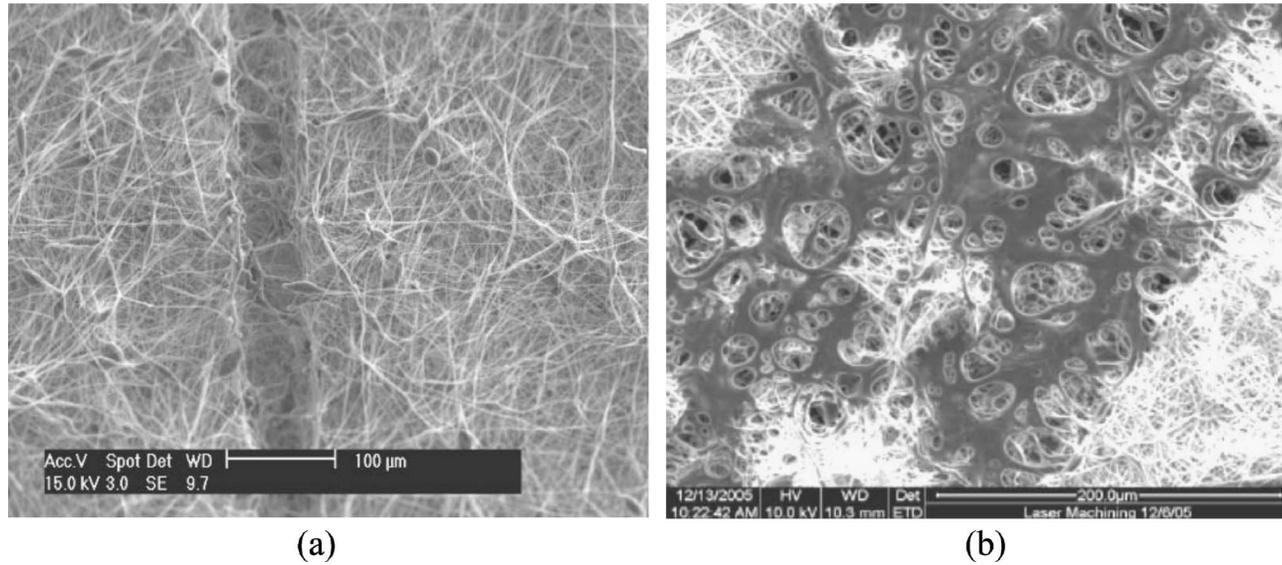
FIG. 7. (a) Focused and (b) defocused (multiple passes, right) scans showing that the lower fluence due to beam defocusing melted rather than ablated the mesh.
