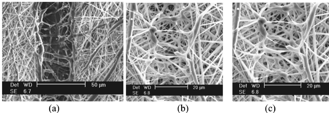
FIG. 6. Two grooves ablated in PCL nanofiber with the 0.1 NA optic at a speed of 20 mm/s and relatively low energy. (a) Pulse energy=1.5  $\mu$ J, fluence=9.3 J/cm<sup>2</sup>; (b,c) pulse energy=0.75  $\mu$ J, fluence=4.6 J/cm<sup>2</sup>.
