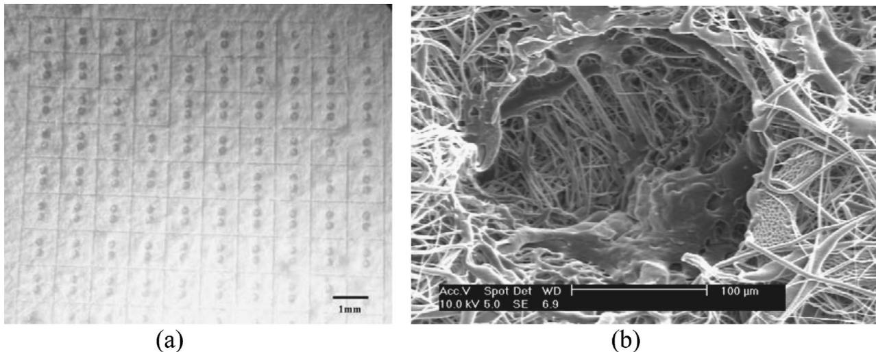
FIG. 10. (a) Matrix of microscale structures ablated in PCL nanofiber mesh and (b) magnified view of a laser-machined cavity in PCL nanofiber mesh (right) begin used in a cell culture test.
