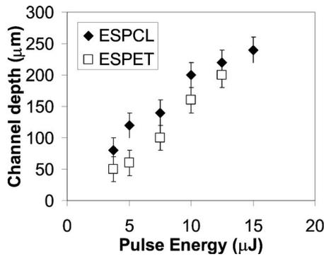
FIG. 4. Depth of grooves machined in ES nanofiber meshes at various pulse energies using the 0.1 NA optic and speed of 20 mm/s showing that PCL grooves were slightly deeper. Error bars indicate error in estimating groove dimension.
