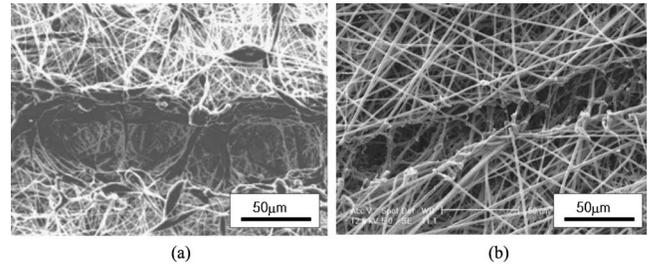
FIG. 5. Comparison of grooves in (a) PCL and (b) PET.
