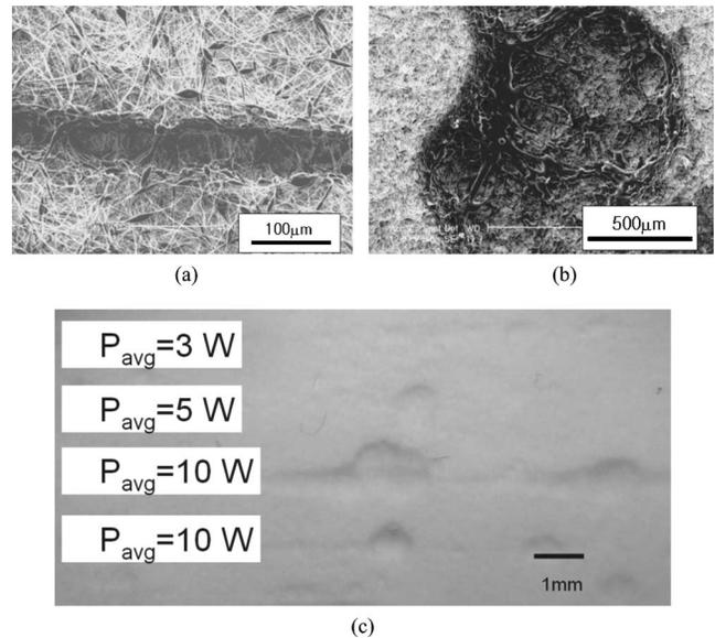
FIG. 2. SEM images of (a) femtosecond laser and (b) Q-switched laser grooves. The width of the femtosecond laser groove is approximately 35  $\mu\text{m}$ . (c) Q-switched laser power was varied from 3 to 10 W, but no power that produced consistent ablation was determined.
