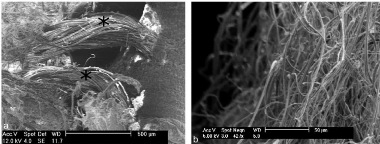
**Figure 10.** (a) Sutures (marked with an \*) stabilizing an electrospun graft (left hand side of image)/tissue (right hand side of image) interface utilizing the procedure given previously. (b) Section of 18 wt% PCL through which the sutures in (a) have been pulled showing a clean failure.
