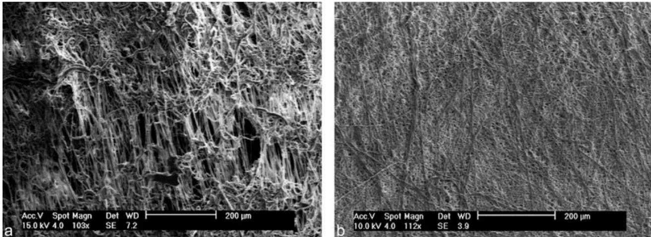
**Figure 8.** Low magnification views of (a) 25 wt % PCL at 45.7% diametric strain and (b) 6.7 wt % PCL HFIP at 42.8% diametric strain. The acetone-based compositions show the pictured localization of stress between braided fiber in between which aligned fibers are visible. In contrast, the HFIP-based composition shows only moderately aligned fiber free of the obvious areas of localized deformation in (a).
