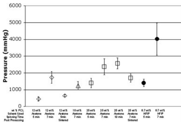
**Figure 6.** Burst pressure versus electrospinning conditions. Only the 25 wt % PCL and 6.7 wt % PCL HFIP cases achieved clinically desirable burst pressures.
