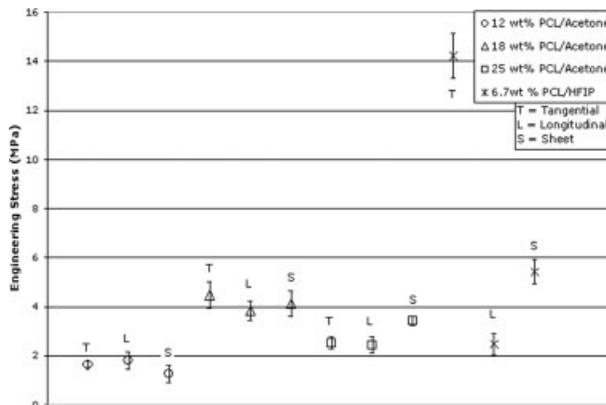
**Figure 1.** UTS of the PCL-solvent compositions. T = tangential (in the direction of the intended orientation); L = longitudinal (transverse to the intended orientation); S = sheet (unoriented).
