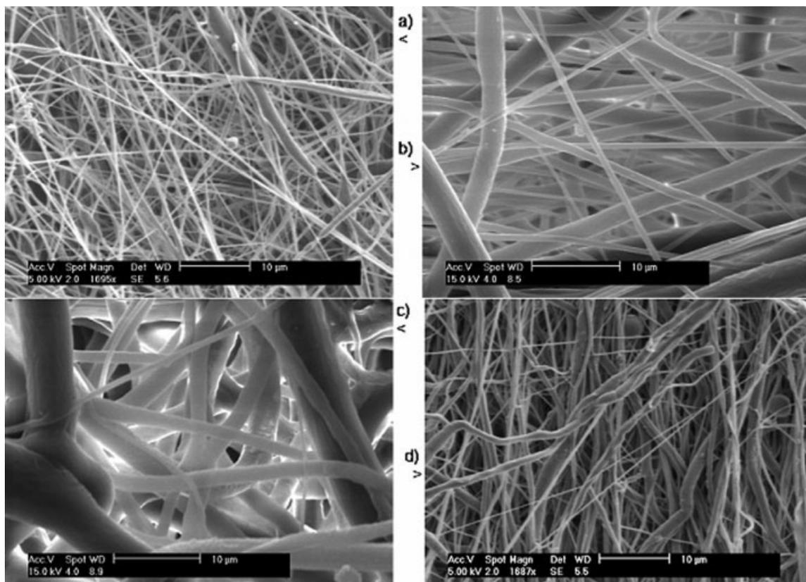
**Figure 4.** SEM images of mandrel-deposited electrospun PCL fibers. a) 12 wt %; b) 18 wt %; c) 25 wt %; d) 6.7 wt % HFIP PCL. The tangential direction is the vertical direction in all but b) where the tangential direction is horizontal.
