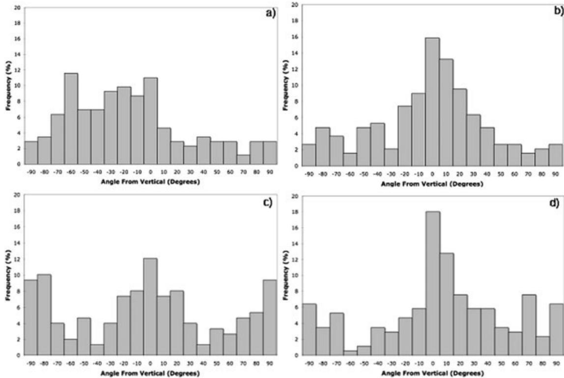
**Figure 5.** Orientational measurements taken from the images in Figure 6 of mandrel-deposited electrospun PCL fibers. a) 12 wt %; b) 18 wt %; c) 25 wt %; d) 6.7 wt % HFIP PCL.
