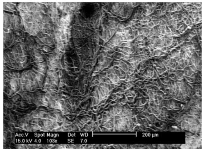
**Figure 7.** A low magnification view of the 18 wt % PCL structure under sustained 41.5% diametric strain. Note the distribution of large and small fiber diameters and the segregation of the larger fibers into braided structures.
