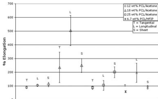
**Figure 2.** Strain data from the PCL-solvent compositions. T = tangential (in the direction of the intended orientation); L = longitudinal (transverse to the intended orientation); S = sheet (unoriented).
