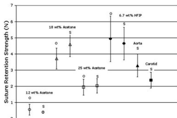
**Figure 9.** Suture retention strengths (S = straight cut; O = oblique cut) for the electrospun compositions versus natural tissues. With the exception of the electrospun 12 wt % PCL can meet or exceed this surgical requirement of matching natural tissues.
