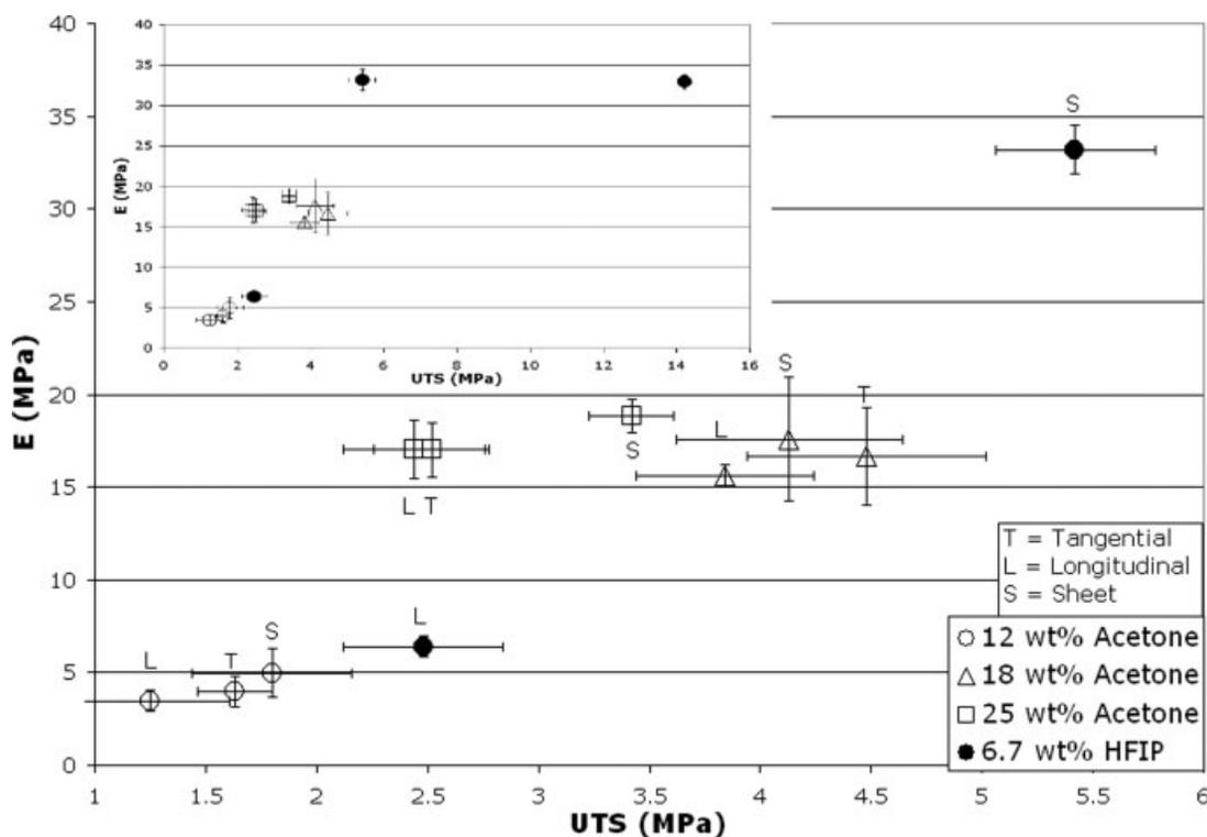
**Figure 3.** Modulus versus solvent identity and solids loading. Acetone compositions (12, 18, and 25 wt % PCL) result in clustering not present in 6.7 wt % PCL HFIP data (see inset) that varies widely. Not surprisingly, the longitudinal direction displays a lower average for 6.7 wt % PCL HFIP. The tangential 6.7 wt % PCL HFIP data is plotted in the upper right-hand corner of the inset) has a modulus identical to the sheet data but its UTS is more than twice as large.
